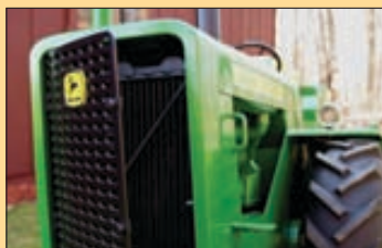
UNIQUE: An access door on the John Deere 8020 reveals the radiator.
