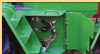
HIDDEN: The light switch and control for the engine sound track are hidden.
