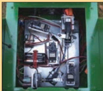
POWER: The servo and electronics are connected to two battery-powered motors mounted in the front.
