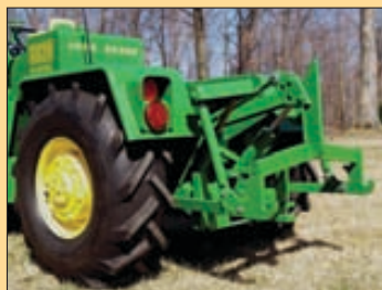
FUNCTIONAL: The three-point hitch is spring-loaded, and the lights work.
